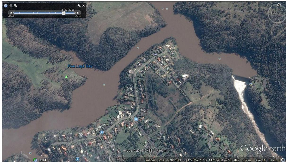
What is apparent from the satellite imagery, is that the intersection of the North and South Esk is not a natural configuration. Intersecting rivers create a Y-shaped confluence which allows the stronger flow to draw out the weaker flowing river and merge side-by-side. It appears that the
