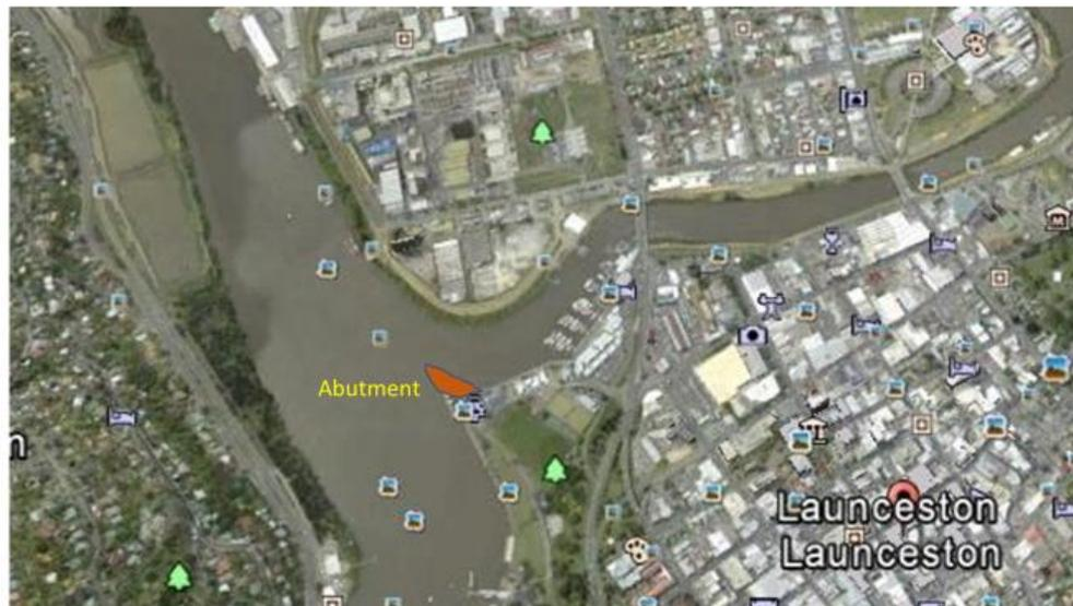
Now, instead of the down-river flow power of the North and South Esk countering each other, they would combine to push against the tidal power of the Tamar and move the silt drop zone further down-river; making it less visually obtrusive.
