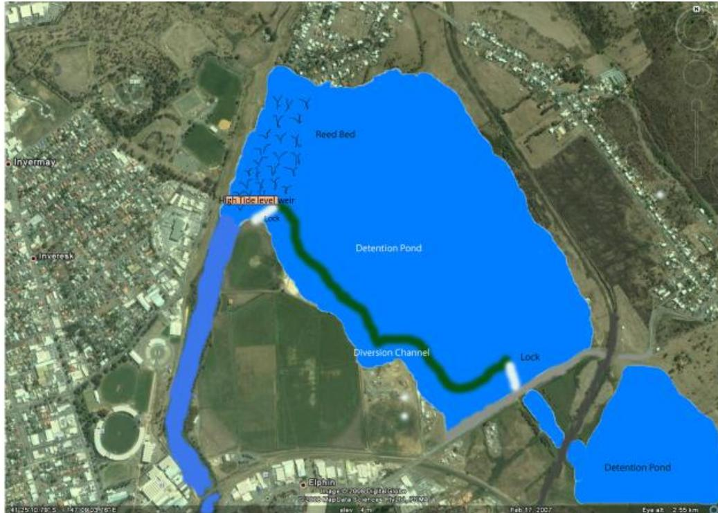
Incorporated within the design would be an ability to drain the pondage when silt level reaches a desired point to allow for its simple dry removal (much as from dredge ponds but without silt plumage from the actual dredging).
